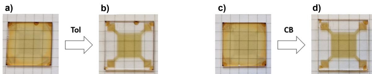
Figure 21. Effect of a toluene and CB exposure on a PCBM layer protected by 10 nm MoO x a) before toluene exposure b) after toluene exposure c) before CB exposure d) after CB exposure.
