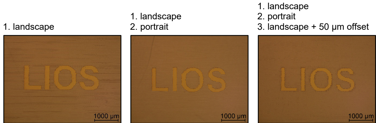
Figure 38. Microscope images of laser patterned ITO substrates (laser power = 20 %, laser speed = 20 %) with successive steps with different laser directions and an offset.
