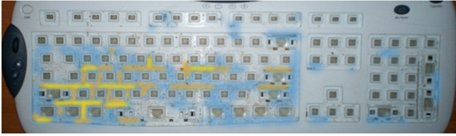
Figure 2: Heat map of the amount of dirt on an opened keyboard. Yellow areas represent peak dirt locations [Tar07]
