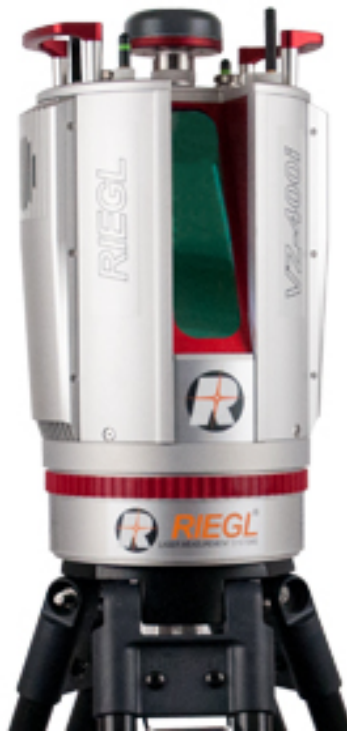
Figure 2.5: 3D scanner used to map the collector shafts.[45]
