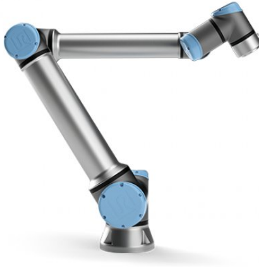
Figure 2.6: The mechanical arm of the robot, where a 3D camera can be mounted for fine-grained inspection.
