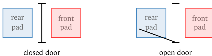
Figure 2.1 Setup for an automatic door (top view): the door in question does not open sideways (like most automatic doors in shopping centers), but towards the rear (like the entrance door to the Open Innovation Center on JKU campus).
